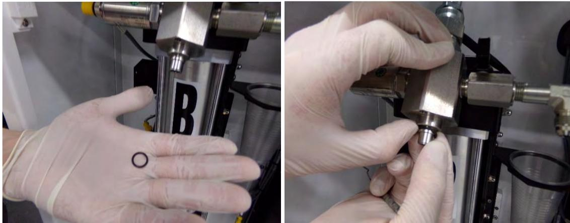
**Figure 17: Replacing the O-ring**
