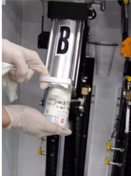
**Figure 10: Removing a Cartridge**
