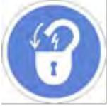
Before performing any repairs or maintenance to the system, turn off power and lock out the power disconnect switch.
