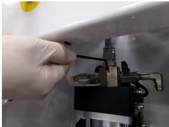
Figure 15: Unscrew Transducer Screws
