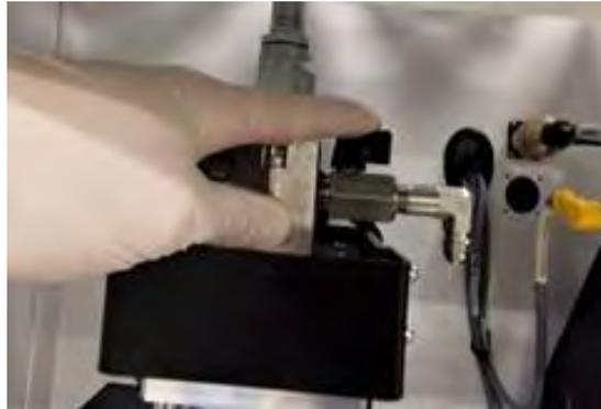
**Figure 13: Opening the Ball Valve**
