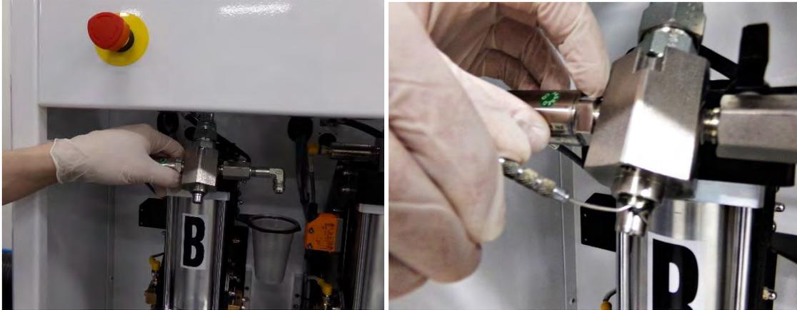
**Figure 16: Removing the O-ring**
