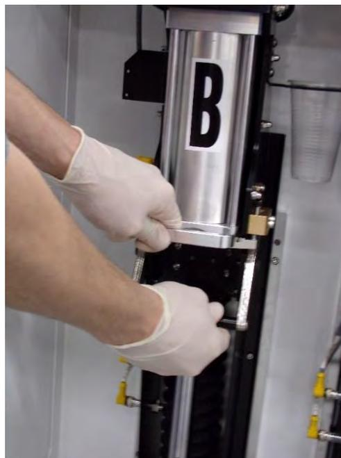
**Figure 9: Releasing a Cartridge**
