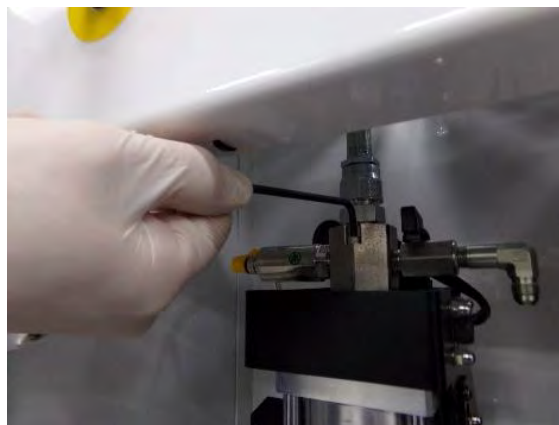
Figure 15: Unscrew Transducer Screws
