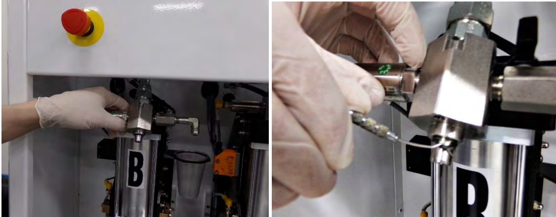
Figure 16: Removing the O-ring
