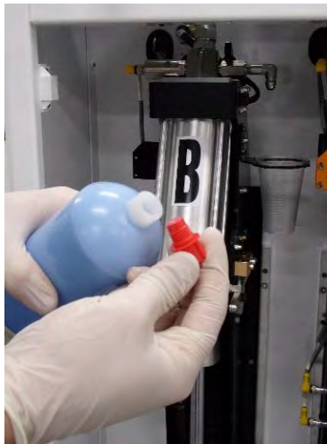
Figure 11: Remove Plug from New Cartridge
