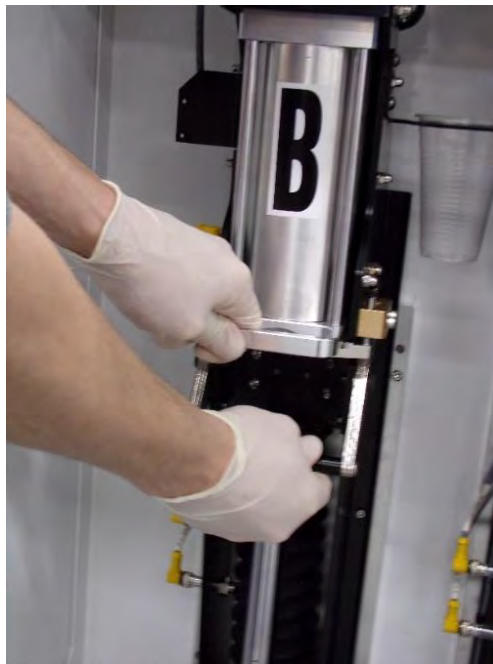
Figure 9: Releasing a Cartridge
