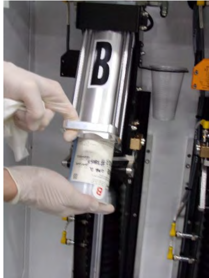
Figure 10: Removing a Cartridge
