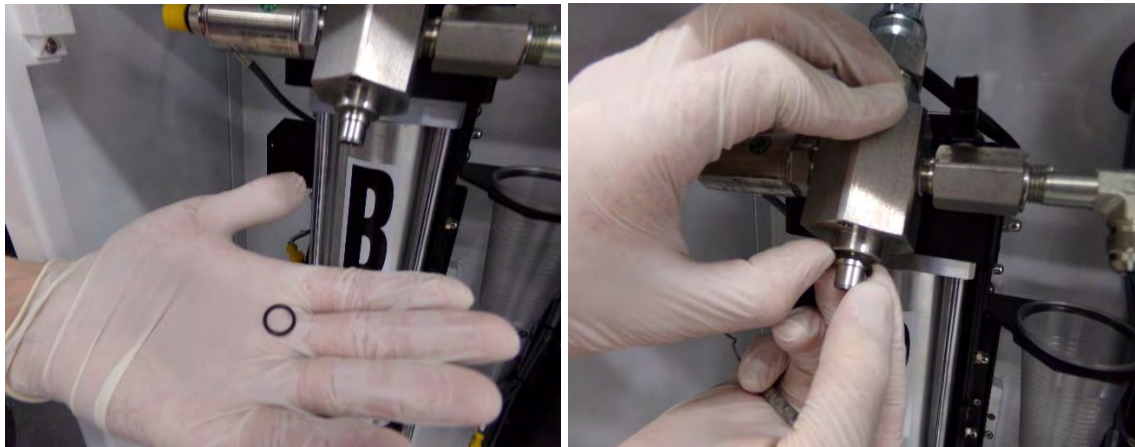
Figure 17: Replacing the O-ring
