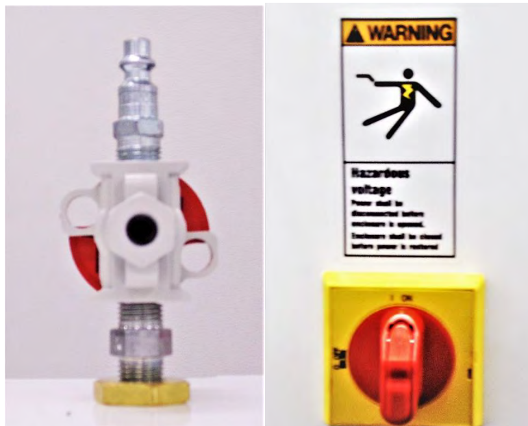
Figure 3: Airline Hookup and Electrical Hookup
