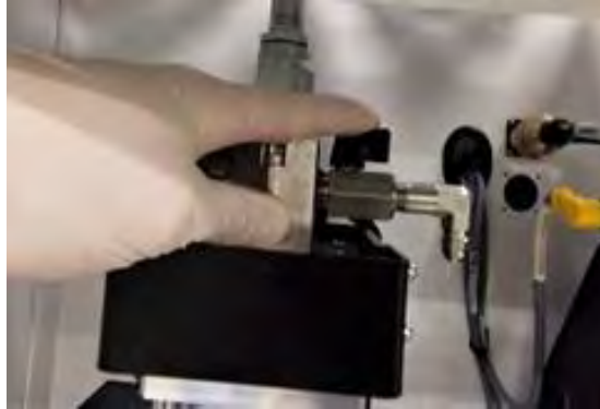
Figure 13: Opening the Ball Valve
